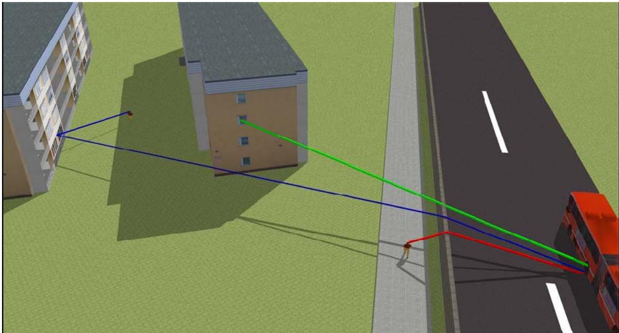
**Fig. Schematic illustration of three scenarios: (1) Outdoors behind barrier at traffic noise exposed side of building (red), (2) Indoors in exposed building (green), (3) Outdoors at "quiet side" of building (blue).**
